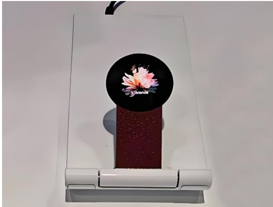
Fig. 3. Photograph of the 1.43-inch in-cell AMOLED display module prototype.
